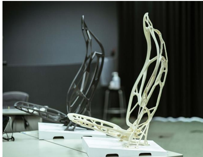
Figure 4. Toyota car seat frame created using GD and 3D printing [30].
